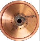
The shield loses its round orifice and sharp edges, becoming oval or with notches.
