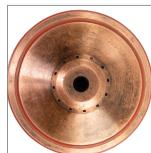
The internal and external orifices are round with sharp edges, and the bleed orifices are not plugged.
