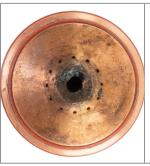
The shield loses its round orifice and sharp edges, becoming oval or with severe notches. This can cause nozzle orifice damage during pilot arc because the arc is not centered.
