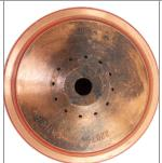
The internal and external orifices are round, and the bleed orifices are not plugged.
